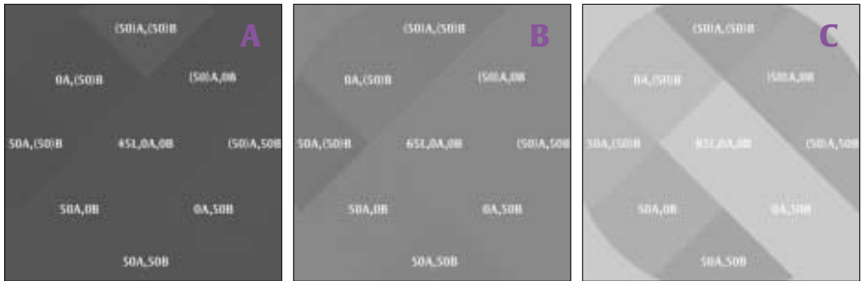
Figure 2.7 The originals of Figure 2.6 had no variation in their L channels. When converted to other colorspaces their luminosity did not remain constant, as Photoshop tried to compensate for the inability to match certain colors. The effect is particularly visible in the lightest of the three versions, where every colored area except yellow has been darkened. These images were converted to grayscale not from the LAB originals, but from the CMYK print files.
