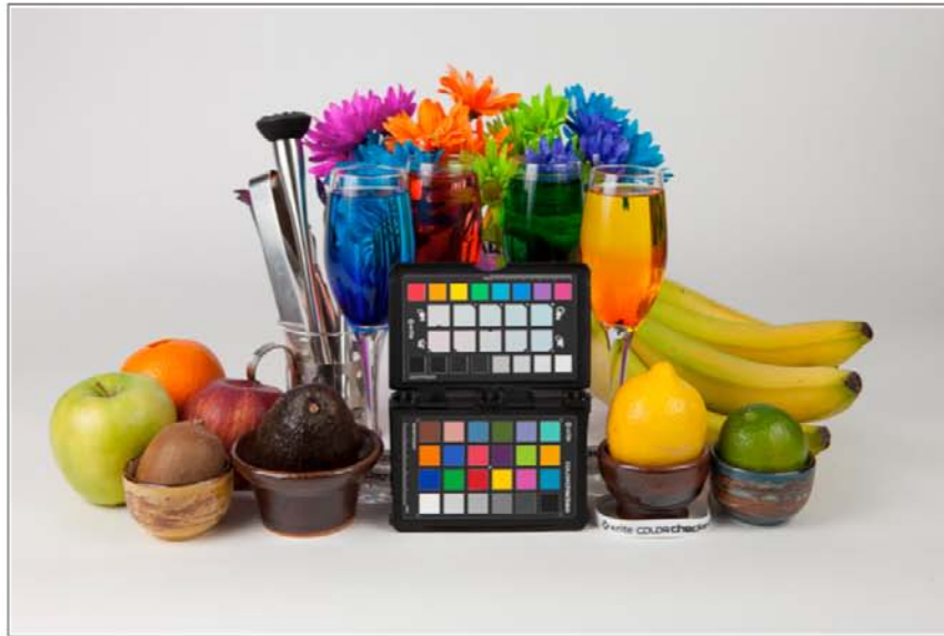
Adequately Exposed. Even steps are visible between each shadow and highlight patch. Black does not go to 0,0,0 and white does not go to 255, 255, 255 (or 100%, 100%, 100%).
